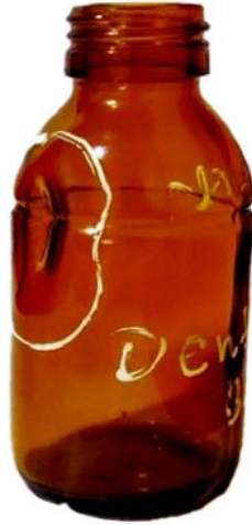
Fig. 1. Defective Container (Dented Body)
